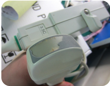
Lens before repair 透镜维修前
